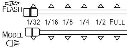
To adjust the PowerLight 1250 to its lowest flash power setting (16 watt seconds), slide the *FLASH* control knob all the way to the left.
